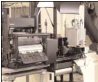
Moveable, slide-out die cassettes increase productivity for folding cartons.
