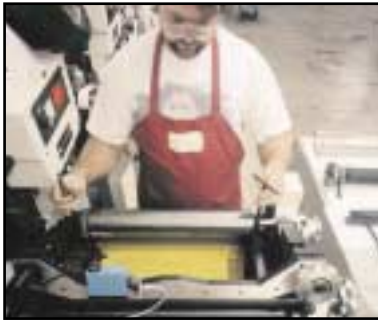
Make-ready idle stations while the press is running.
